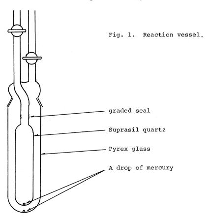
The inner tube is made of Suprasil quartz which is transparent for the UV-light at 253.7 nm even after the f-irradiation. The transmission was 92 % at 253.7 nm. The outer tube is made of Pyrex glass. The joint attached to the outer tube is for annealing the Suprasil quartz tube irradiated by f-rays; however, the transparency at 253.7 nm was not changed even after f-irradiation. At the shorter wavelengths, the transparency was reduced by f-irradiation.
